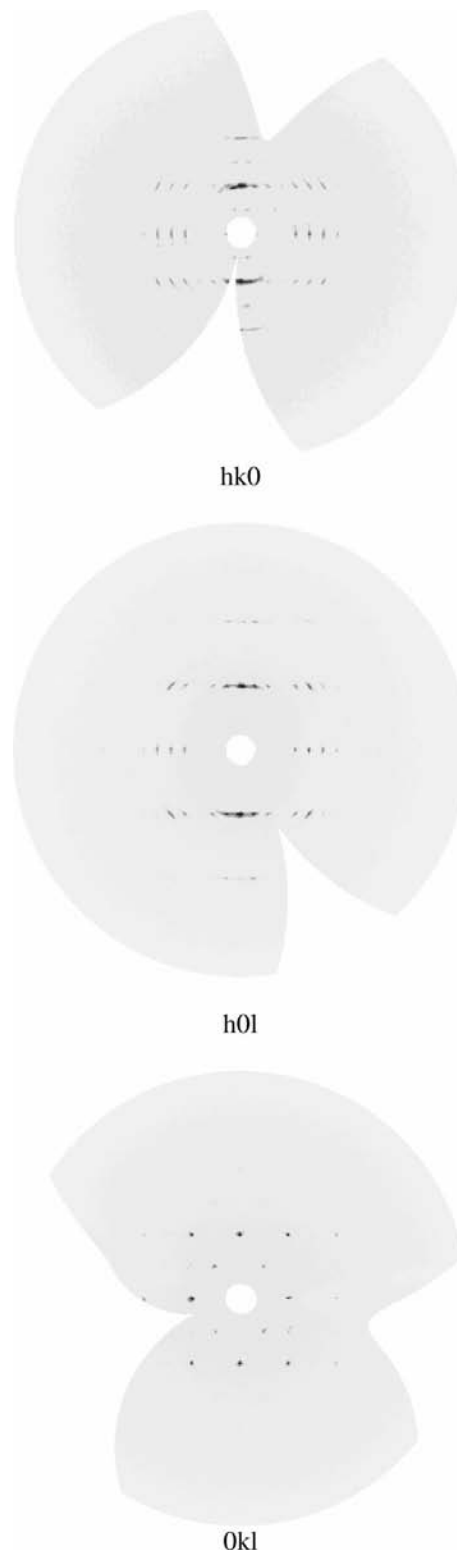
Figure 1 Reconstructed view of the three principal zones of reciprocal space for a crystal of (I).
